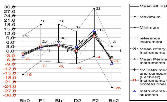
5.1.2 Intonation of the reference trumpet. The fundamental frequency of the a1 blown on the reference instrument depends on the dynamic and varies greatly between players. [illustration: the mean, maximal and minimal values played during a crescendo of the a1; (moment of attack; sustained ppp, the individual minimal amplitude; mf (measured 90 dB); forte (measured 100 dB) and at fff, the individual maximal amplitude).]
