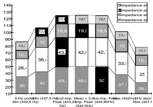
5.1.4 Variations between players. The intonation difference at mf (measured 90 dB) is 58 cent (min.=438 Hz; max.=453 Hz) and at f (measured 100 dB) is still 56 cent (min.=437, 6 Hz; max.=452 Hz)! The influence of different temperatures (18°C-23°C) during the recording cannot be the reason for the variations, since it alters the intonation to a maximum of 15 cent. The differences are caused by the player [ply].
