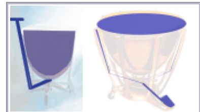
Fig. 2b: Hand tuning mechanism of the Viennese Timpani (left) and the "standard timpani" (right) with a pedal
